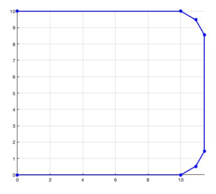
• VLRadiusC for inserting points to generate radial curves instead of corners.
