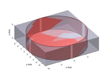
bs=SGsize(nSG); [BB.VL,BB.FL]=VLFLofBB(bs); SGplot (BB, 'w'); VLFLplotlight(1,0.4);
