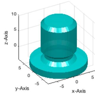
The warnings 'Removed n(m) facets' can be ignored. These warning appear if a part of the contour touches or crosses the  $x=0$  line (y-axis).
