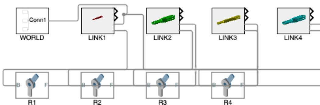
The model of link4 is extended by a transformation sensor
