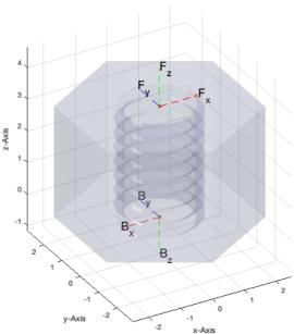
Realization of rotating joints by means of a screw connection DIN 912 and DIN 985
