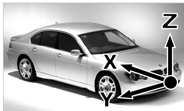
Figure 3.4: Body coordinate system
