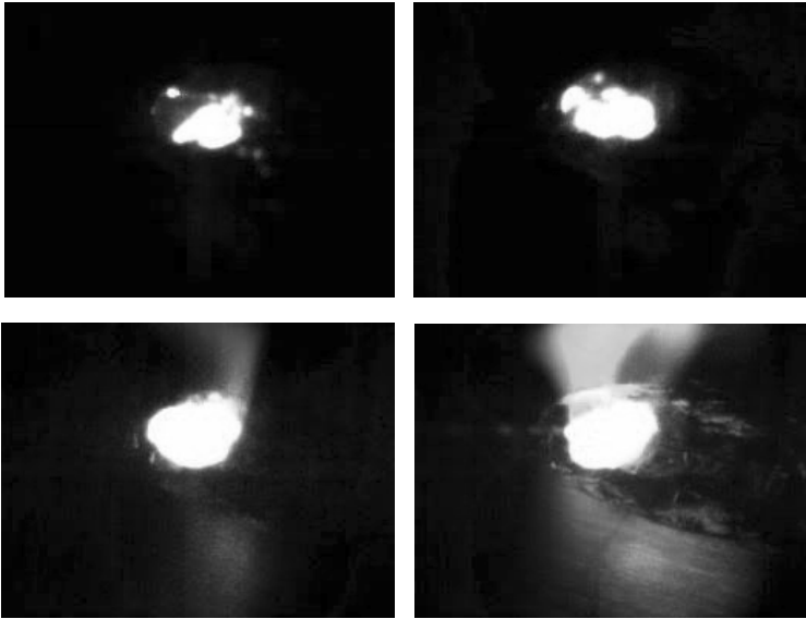
Figure 4.12: Oxide layer obstruction in Nd:YAG laser welding: series of subsequent high-speed photography snapshots; bead on plate; EN AW-6060; 10000 fps; P_{Nd:YAG} = 3 \text{ kW} ; f = 200 \text{ mm} ; \phi = 15^\circ ; argon flow 25 \text{ L min}^{-1} ; v_w = 2 \text{ m min}^{-1}
