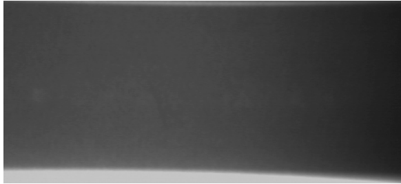
Figure 5.31: Surface-on x-ray transmission photograph of BHLW bead with the double coaxial nozzle system; P_{BHLW} = 3 \text{ kW} + 3 \text{ kW} ; f = 150 \text{ mm} ; \phi = 6^\circ ; v_w = 3.0 \text{ m min}^{-1} ; bead on plate; EN AW-6060; inner nozzle: helium flow 9 \text{ L min}^{-1} ; helium flux 2.9 \text{ L min}^{-1} \text{ cm}^{-2} ; outer nozzle for guiding gas: argon flow 10 \text{ L min}^{-1} ; argon flux 2.8 \text{ L min}^{-1} \text{ cm}^{-2}
