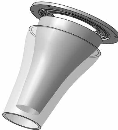
Figure 5.6: Exploded drawing of the double coaxial nozzle system and the injection plate; the outer nozzle was made transparent to show the inner nozzle
