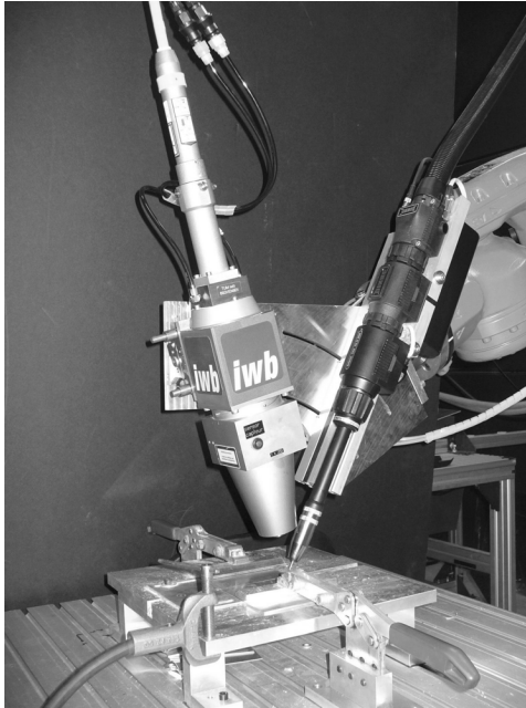
Figure 3.6: Experimental head for laser augmented MIG welding; MIG torch arranged in pushing backward position with regards to laser spot
