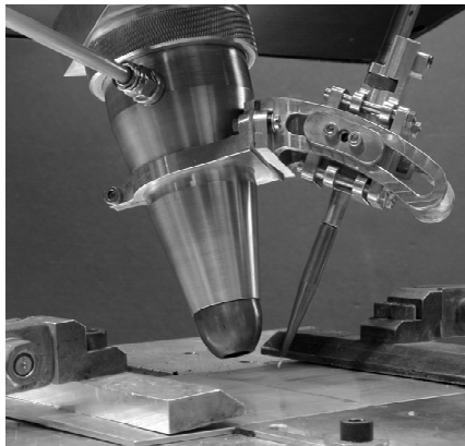
Figure 8.15: Filler wire supply unit mounted to a conical gas nozzle on the bottom of the experimental optic setup
