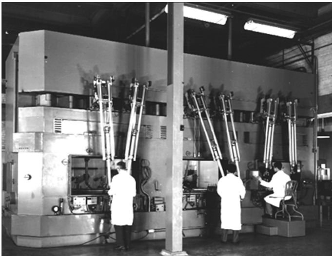
Figure 2.2: The first teleoperation system for handling nuclear materials
