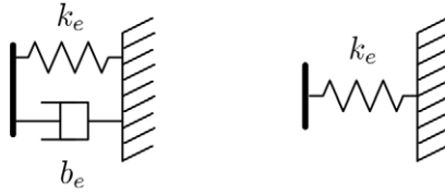
Figure 4.10: Schematic representation of a viscoelastic environment (left) and a pure elastic environment (right)
