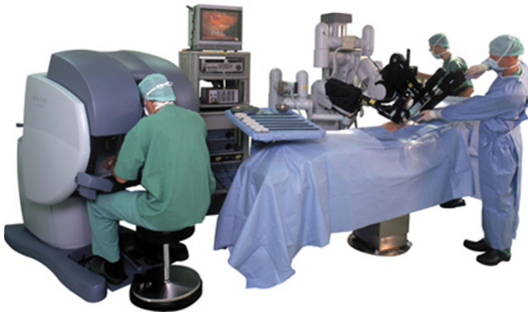
Figure 2.3: da Vinci®: the telepresence system for performing minimally invasive surgery (INTUITIVE SURGICAL 2011)
