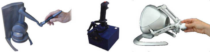
Figure 2.6: Examples of haptic devices available in market: PHANTOM Desktop from Sensable (left), Impulse Engine 2000 from Immersion Corp. (middle) and Falcon from Novint Technologies Inc.(right)
