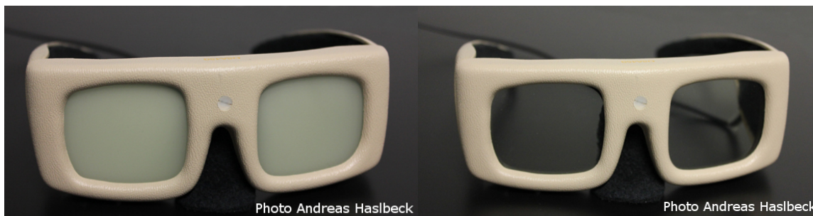
Figure 1 Shutter glasses (PLATO, Translucent Technologies, CA) open typically 1.5 seconds and closed typically 1.5s (ISO 16673)
