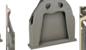
TopOpt with improved constraint formulation
