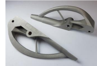
Gripper for a handheld screwdriver by STÖGER AUTOMATION GmbH: The support-free redesign (right) provides mass savings of 30% compared to the conventional design (left).
