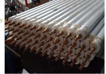
Current generation muon detector tubes at a partner institute
