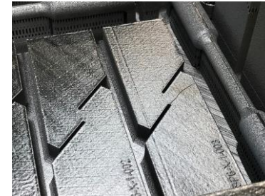
Crack in AM specimen
