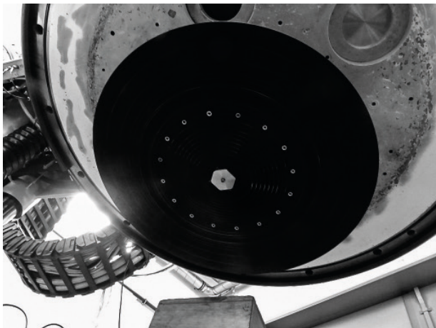
CFRP disk mounted on a spin test stand
