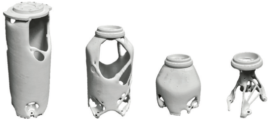
Fig. 2: 3D printed optimized parts from Link1 (left) to Link4 (right)
