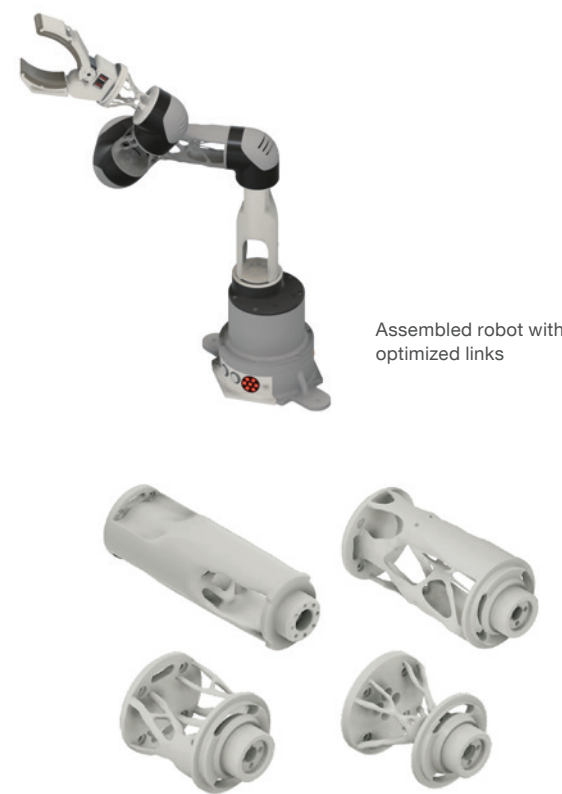
Topology optimized robotic structures subject to dynamic loads
