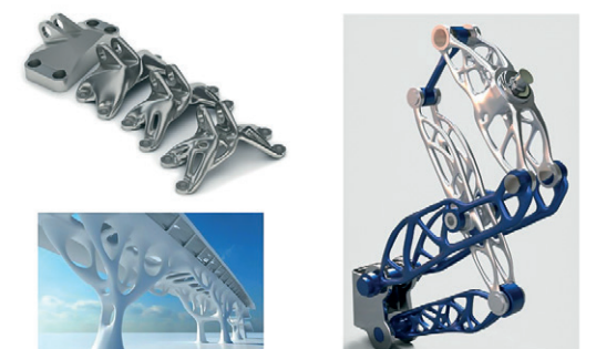
Fig. 1: Applications of topology optimization: from single parts to complex systems and large-scale structures. © DTU
