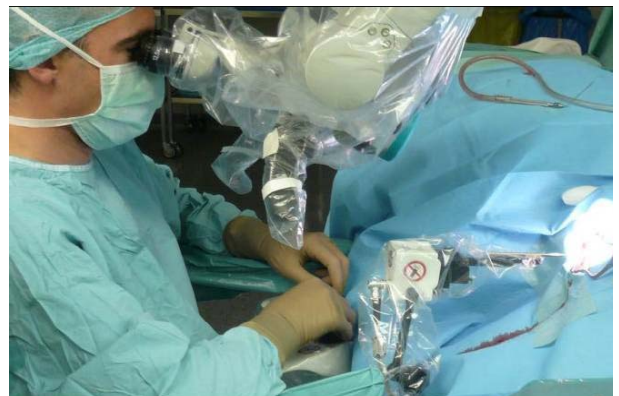
Fig. 9. Placement of the MMS-II at the side rail of the OR table.
