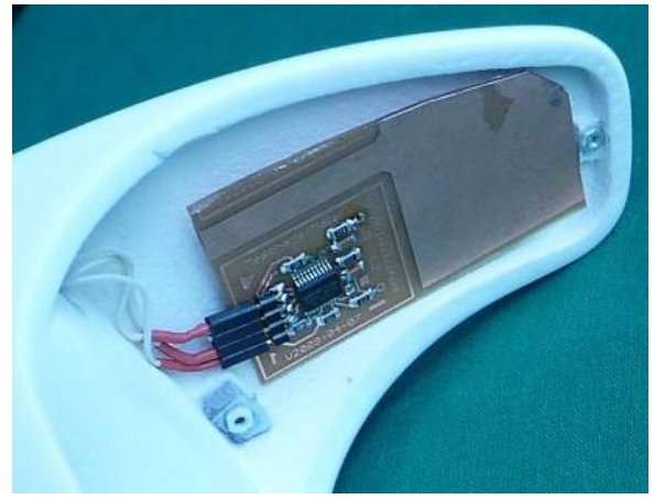
Fig. 8. Capacitive sensor IC together with sensor area in the hand rest.
