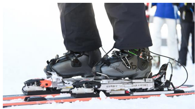
Specially built measuring ski binding to record all occurring forces and moments during skiing.
