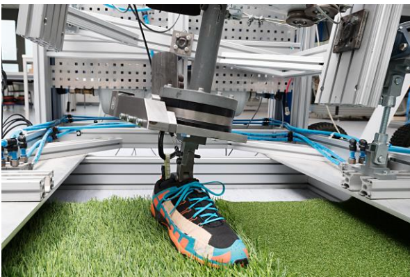
A traction measurement for trail running shoes is performed on the TrackTester
