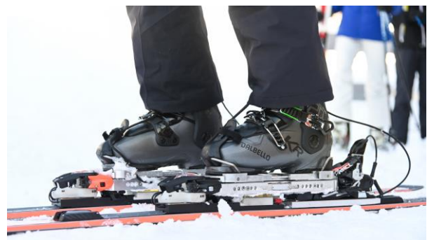
Specially built measuring ski binding for recording all forces and moments that occur during skiing.
