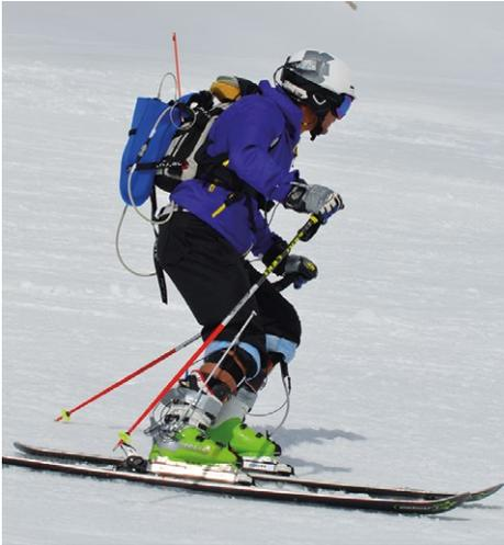
*Instrumented skier with dynamometers, goniometer, differential GPS and inertia sensors*
