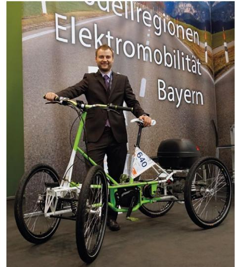
Four-wheel electric bicycle 'QuadRad' with heart rate controlled support
