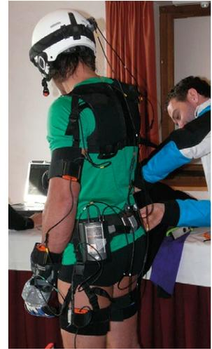
*Attaching and wiring the inertia full body motion capture system*
