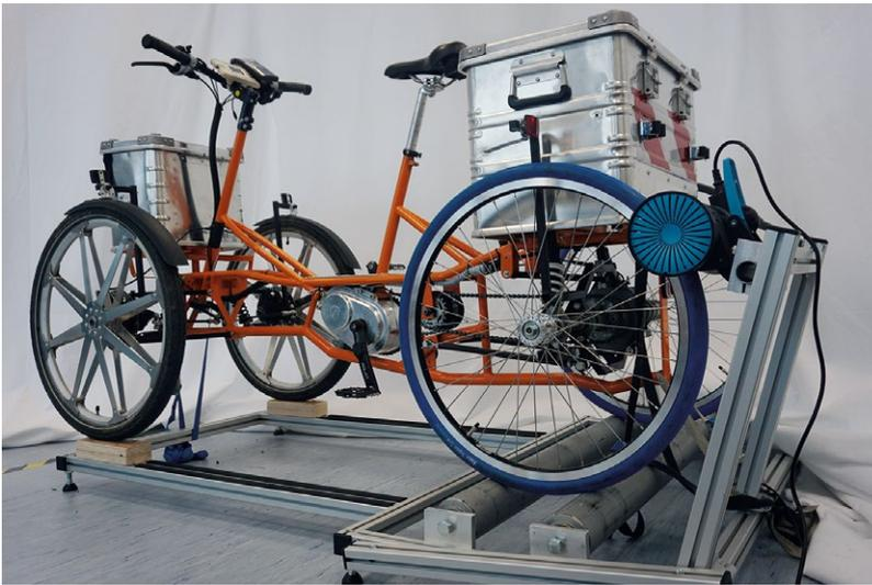
Prototype 'QuadRad', a new category of electric driven lightweight vehicle, on the test bench
