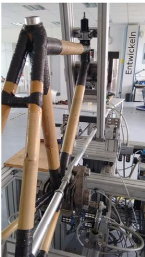
Bamboo bicycle frame during fatigue tests
