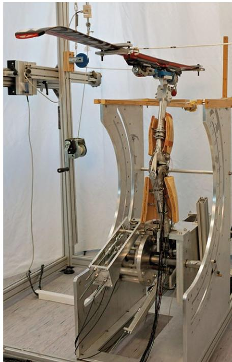
*Artificial surrogate leg with load application unit for the development of mechatronic ski bindings and knee protectors*
