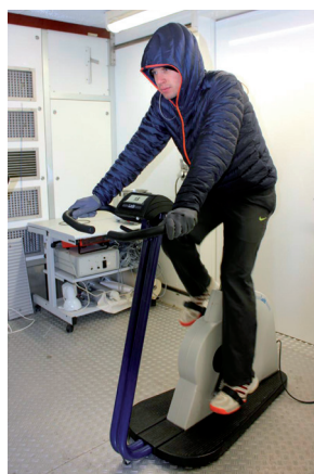
Skin- and core temperature measurements during garment test in climate chamber
