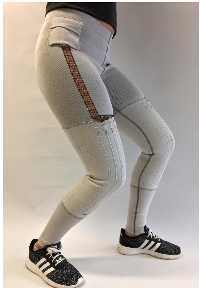
Ski underwear with textile integrated sensors to measure knee flexion angle
