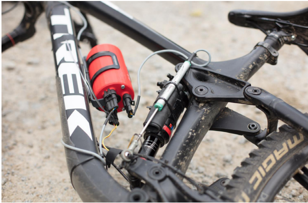
Data logger and linear displacement measurement at rear suspension (photo: Lars Scharl)
