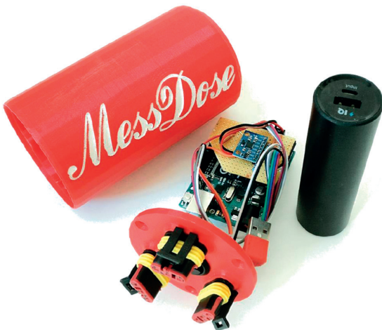
Custom built data logger to measure cycling speed, displacements and velocities at the suspensions, three axis accelerations, angular displacements and velocities
