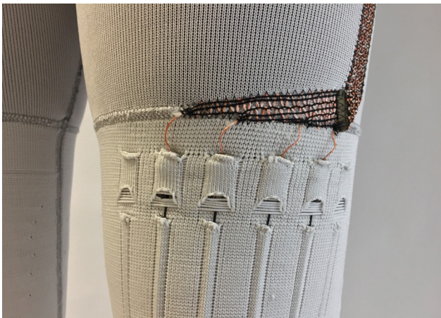
Ski underwear with textile integrated sensors to measure knee flexion angle
