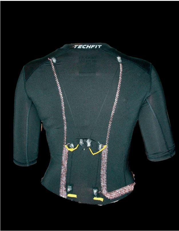
Sensor shirt with measuring fibres (TUM)
