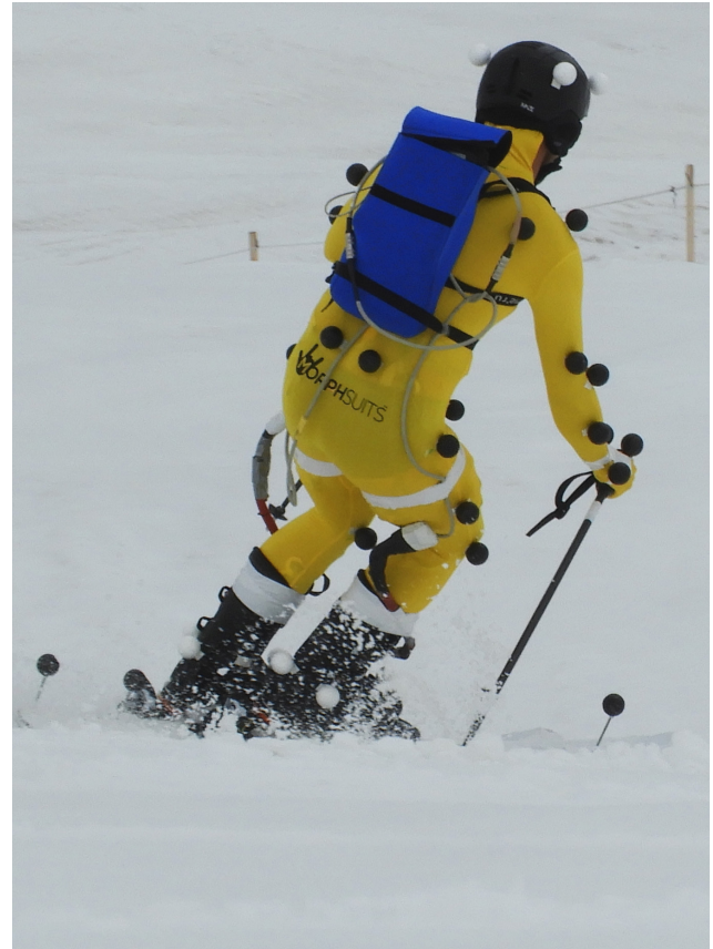
Skier with skin-mounted markers for video-based 3D-motion analysis (Source TUM-SpGM)
