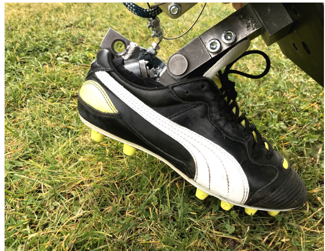
Mechanical foot model of the TUM TrackTester to reproduce a realistic load pattern between shoe and turf
