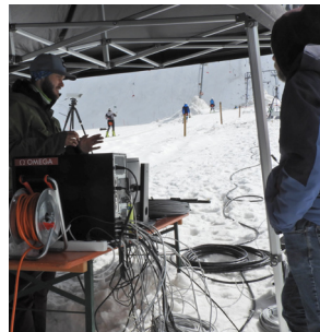
Field Study at Stilfser Joch/Italy setting up 16 cameras and performing the calibration of the observation space (Source: TUM-SpGM)
