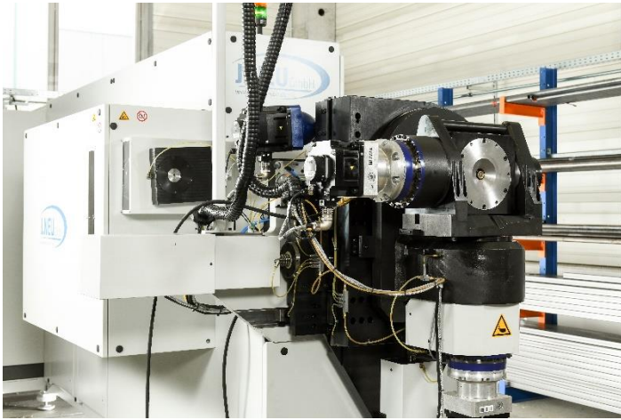
Figure 1: Freeform bending machine with six simultaneous axis.
