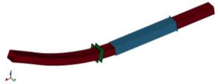
Fig. 2 Simulation model of a rectangular tube
