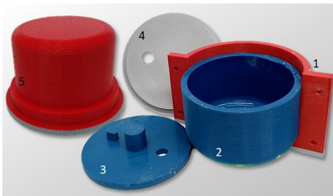
Abb. 1 Indirect Rapid Tooling approach; casting mold with hard mold (1), silicone mold (2), silicone lid (3), FDM lid (4) and FDM mold negative (5)
