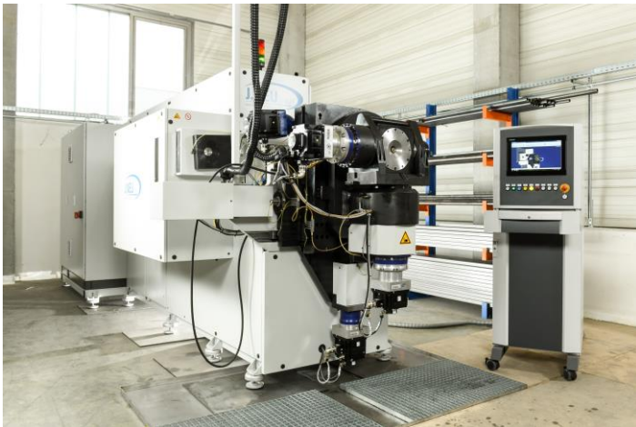
Fig. 1: Free-form bending MOS machine by J.Neu GmbH
