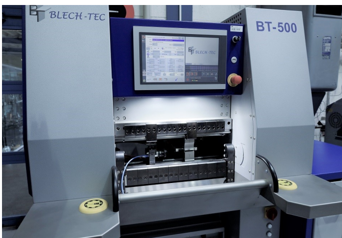
The Compact Bending Machine BT-500 from Blech-Tec for Small Sheet Metal Parts, Photo: utg
