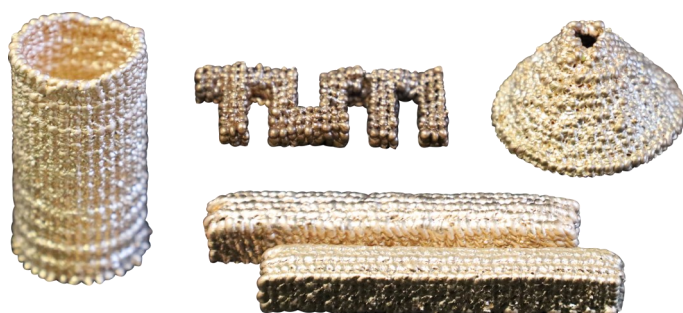
Fig. 1: MJT Additively Manufactured Components made of Pure Copper and Bronze, Photo: utg
