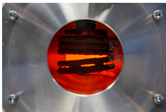
Fig.2: Heating Chamber with Induction Coil, Photo: utg
