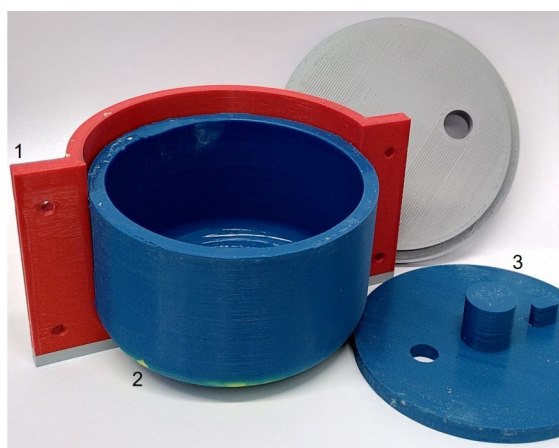
Fig. 1: Mold According to Indirect Rapid Tooling Approach, Photo: utg
