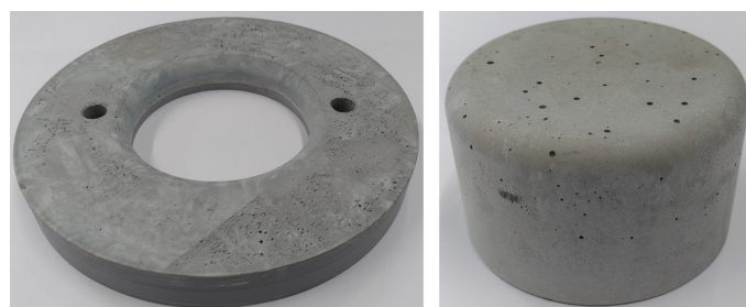
Fig. 2: UHPC Tool Die and Punch, Photo: utg
