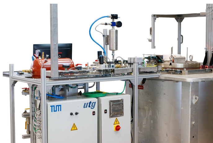
Fig. 1: Low-pressure casting system for casting asynchronous rotors, photo: utg
