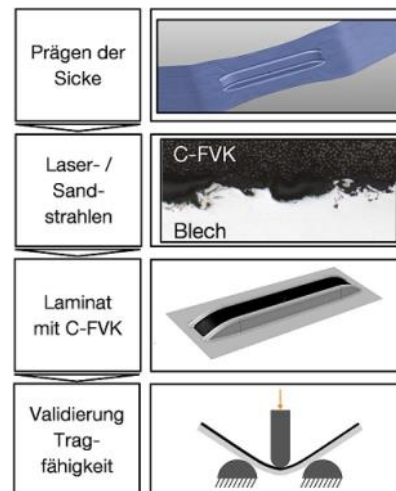
Steps for manufacturing and validation of the Hybrid Beads, Image: utg & IPEK
