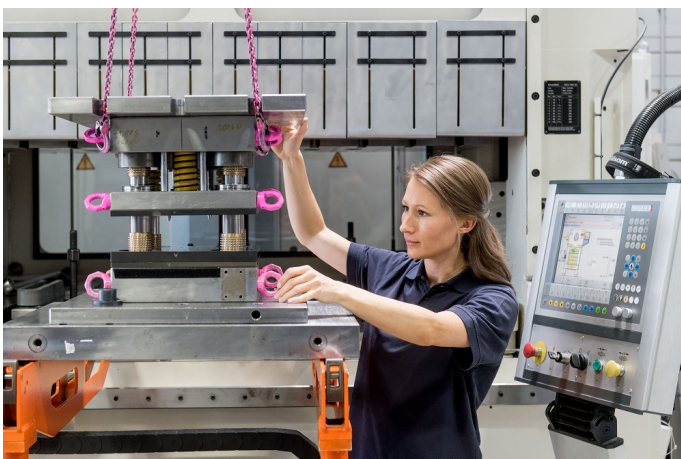
Isabella Pätzold installing Tools on the Bruderer Press, Image: Hase/utg
