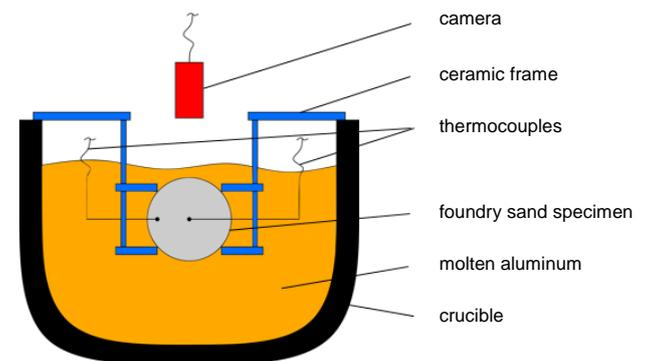
Fig. 2: Principle sketch of the setup for determining the temperature profile in inorganic molding material during casting.
