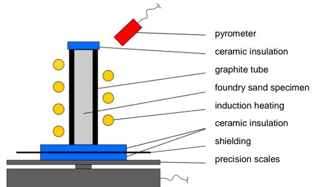
Fig. 1: Principle sketch of the setup for determining the temperature-dependent gas evolution of inorganic molding materials
