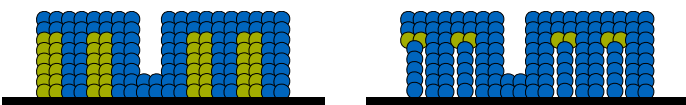
Figure 2: Left: Monolithic salt support structure. Right: release layer support structure. (Kirchebner et al., 2023)
