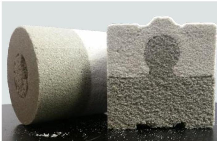
Figure 1: Multilayer core made of two different sand-binder systems, produced in two steps on a core shooting machine.
